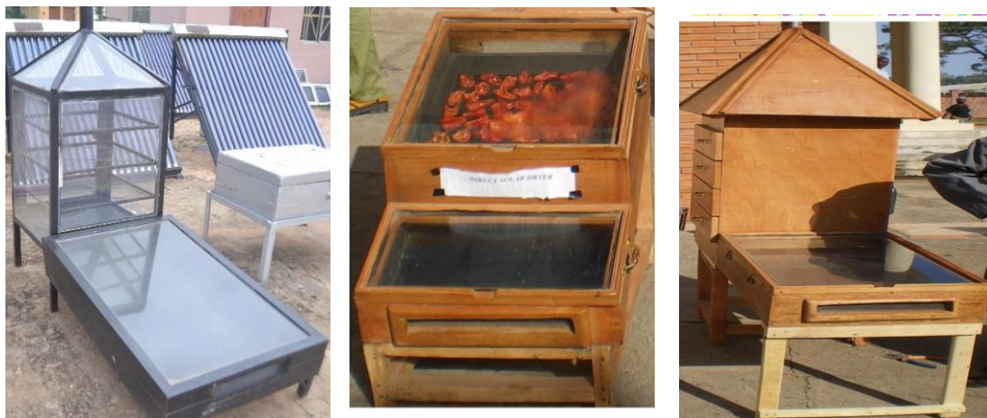
Solar Dryers: Combined mode; Direct and Indirect Types for Domestic Applications
