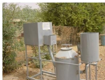
Portable Biogas digester
