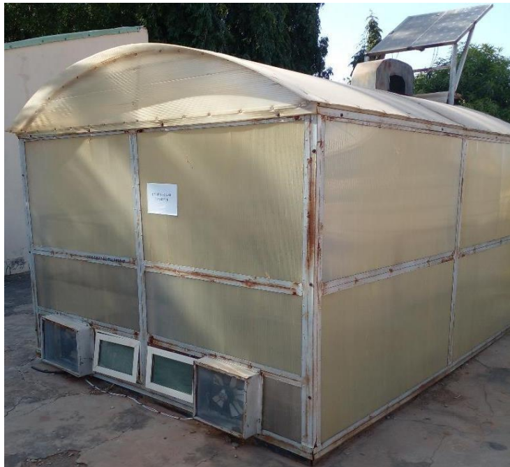
Hybrid-(Active/Passive) Large Scale Solar Dryer
