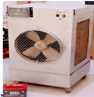
Solar-Powered Evaporative Cooler (Desert Cooler)
