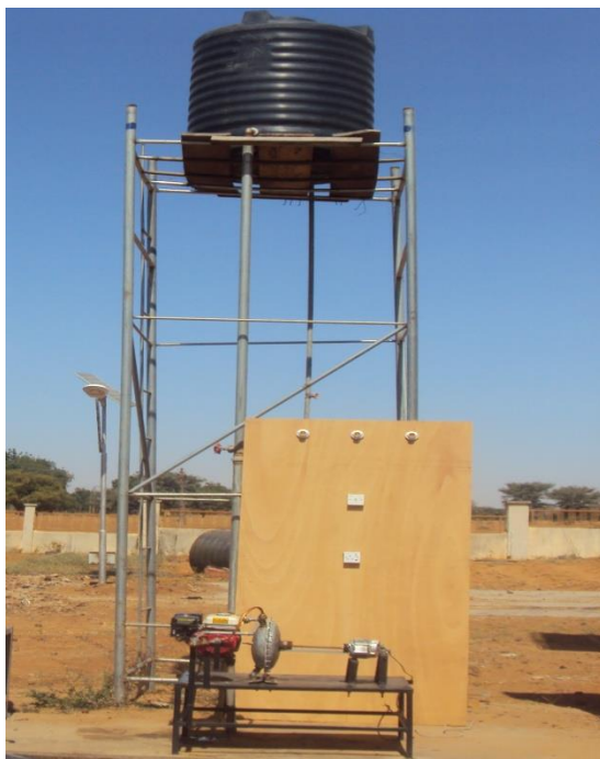
SHP Demonstrating System Locally Fabricated at SERC Demonstration Area
